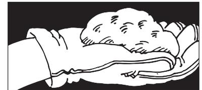
handling and movement. Maintain pressure on the plug with your gloved hand, trowel, or wood block until the EASY PLUG® has set firmly. Keep the EASY PLUG® damp for 15 minutes.
