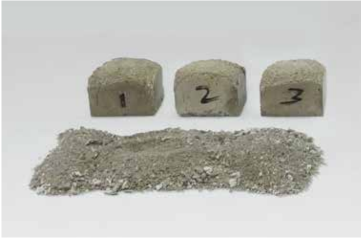
Mortar Mixed With Water after 25 cycles of Freeze/Thaw Testing
