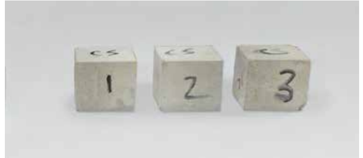
Mortar Mixed With CONCRETE SUPPLEMENT™ after 25 cycles of Freeze/Thaw Testing
